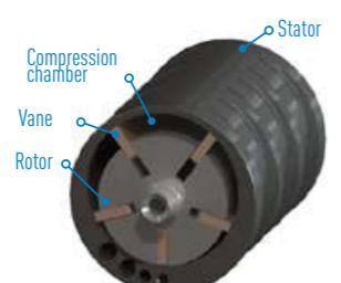
Since the two sides of the chamber made of the two vanes (P1) and (P2) have different surfaces, the force applied onto each of them is different and a rotation motion is generated on the rotor.
